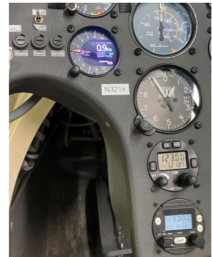
Figure A. N321K Battery 1/2 Switch, Vario, Radio, and Transponder
