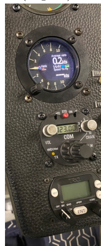
Figure B. N321K transponder, Radio and vario in instrument panel.
