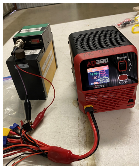
Figure C. Battery and Battery Discharge Setup.
