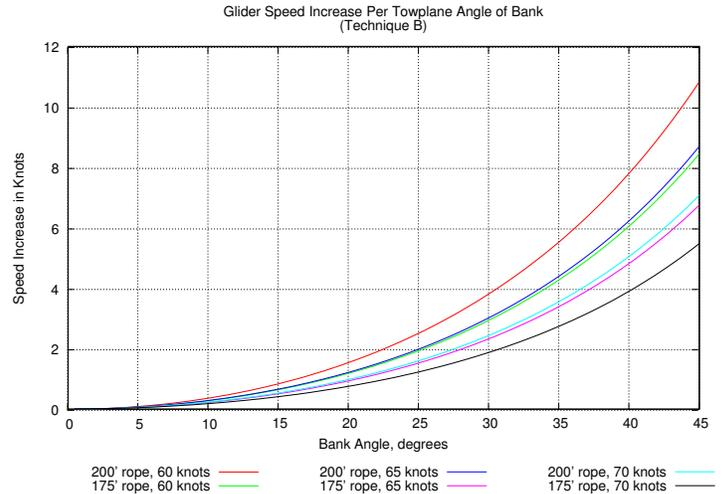
Figure 5: Technique B Glider Speed Increase
