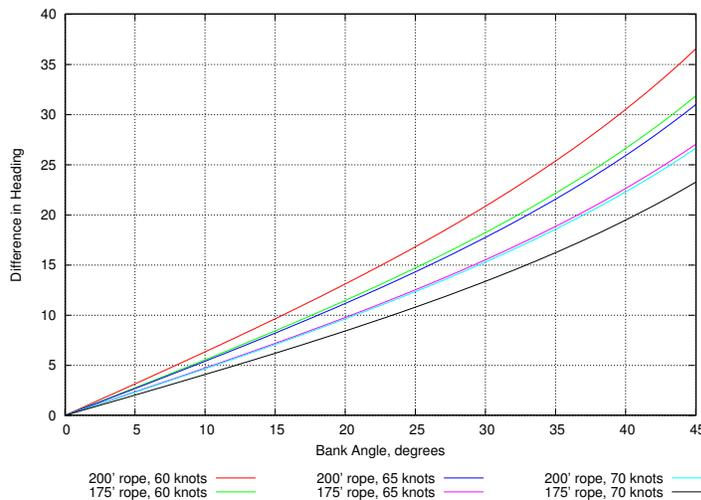
Figure 3: Difference in Heading per Angle of Bank (Technique "A")
